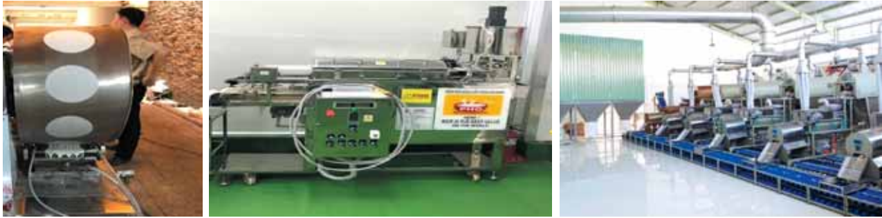
Equipment for the automatic manufacture of rice paper; Equipment for the manufacture of pho and vermicelli; Cashew processing line (from left)
