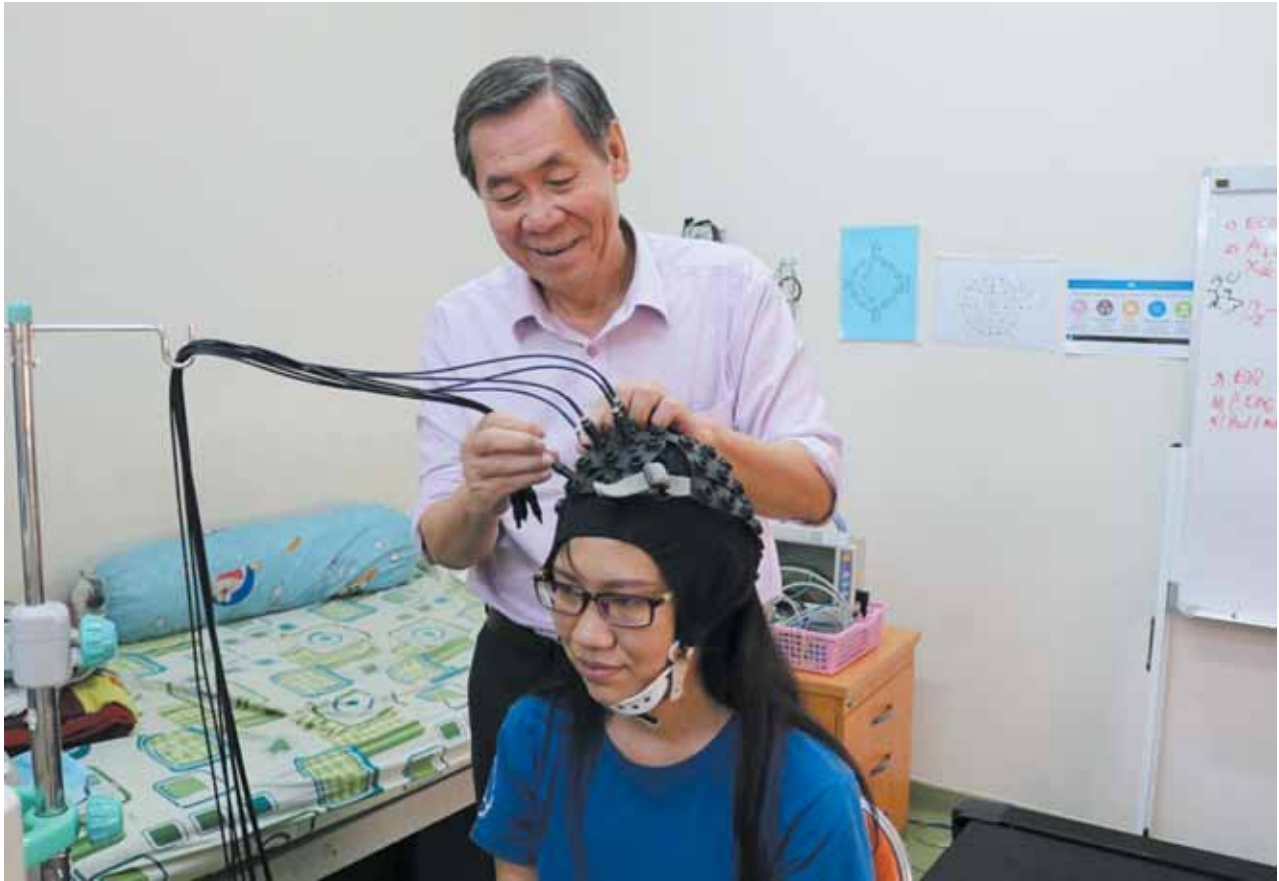
Prof. Dr. Vo Van Toi instructs the students on using functional near-infrared spectroscopy (fNIRS).
